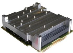
The solution designed by Syrlinks, referenced as the EWC27, brings key advantages such as compactness to fit into nano/cube sats, in-space proven technology (high heritage) and high performances low power consumption, efficient RF transmission, 100 Mbps data rate). Up today, more than 120 flight models have already been delivered.
